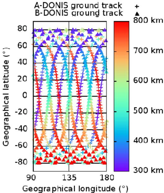
Figure 2: Coverage of the ADONIS mission. Longitude shown from 80 to 180°. The coverage is identical for other longitudes.
