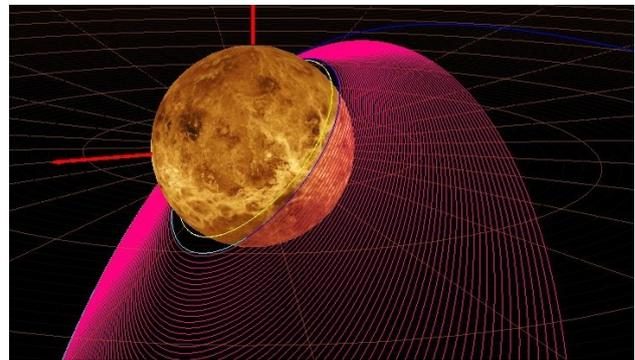
Fig. 4— Venus approach orbit: the arriving hyperbola (blue) the aerobraking (purple) and the final scientific orbit (yellow).
