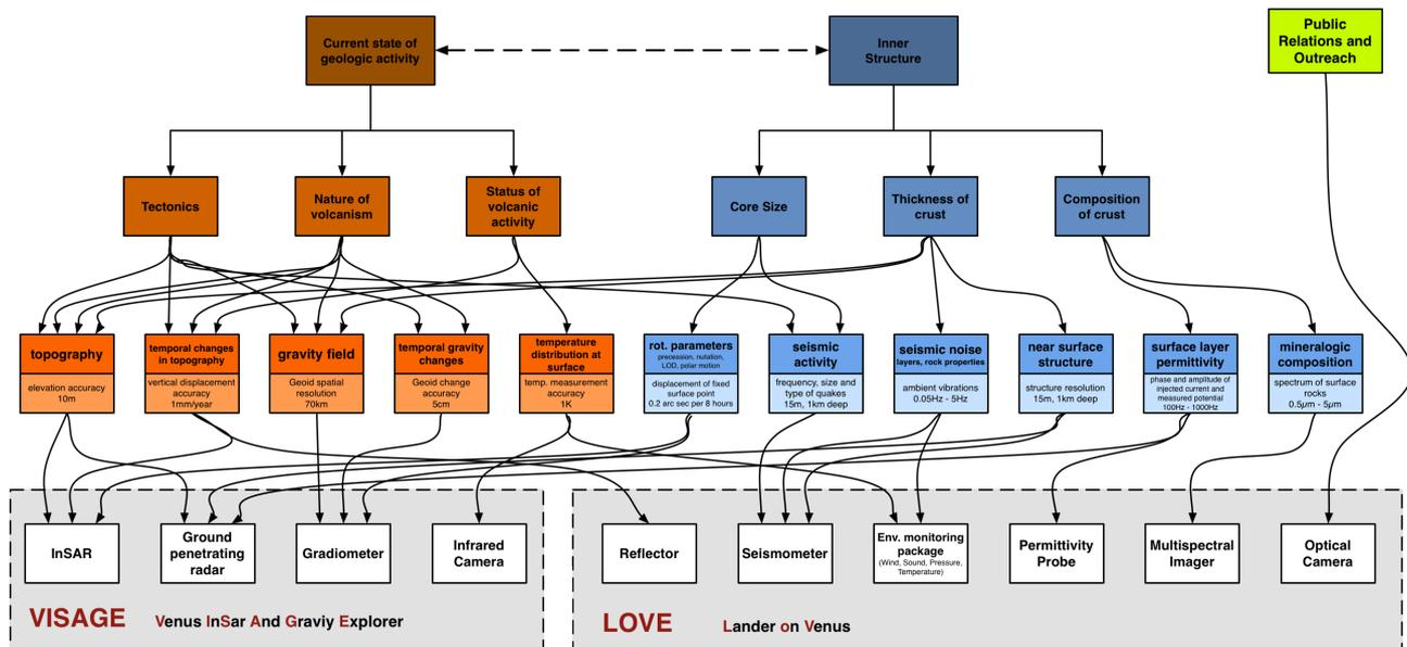
Fig. 2— Flowchart showing connection between scientific objectives, mission requirements and instruments
