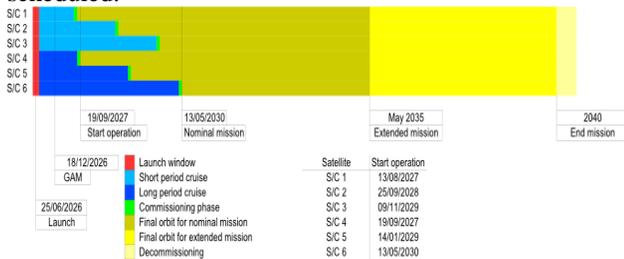
**Figure 13 - Launch and full orbit phases**
