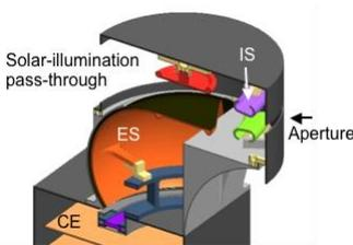
Figure 6 - PAS Cross Section
