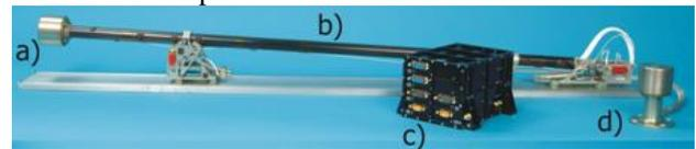
Figure 7 - Magnetometer with Sensor 1 (a), Boom (b), Controller Electronics (c), Sensor 2 (d) from Zhang et al. (2005)
