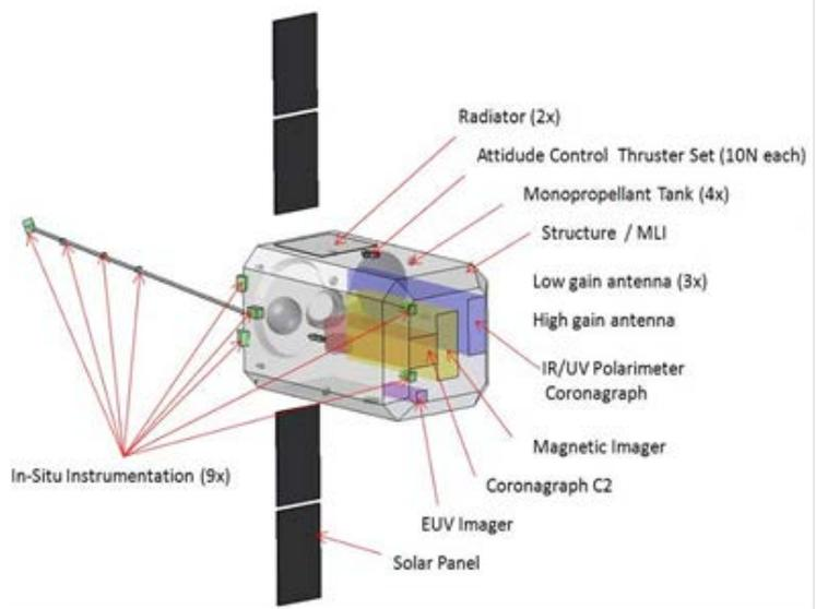
Figure 5: 3D model of the SCE
