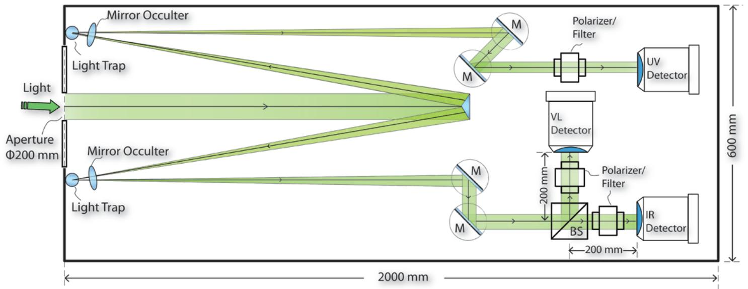
Figure 3: Schematic of the IR/UV Polarimeter
