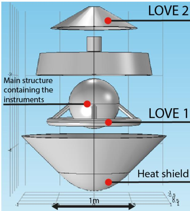
Fig. 6— Main structure of the landing module showing the heat shield and the two landers
