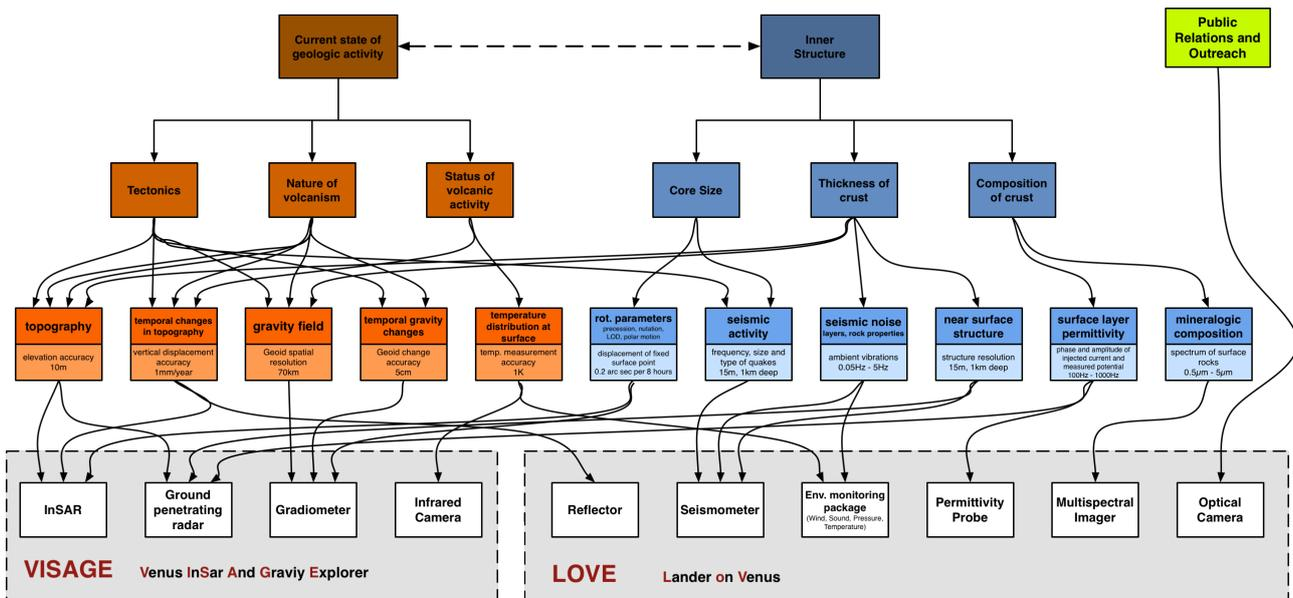
Fig. 2— Flowchart showing connection between scientific objectives, mission requirements and instruments
