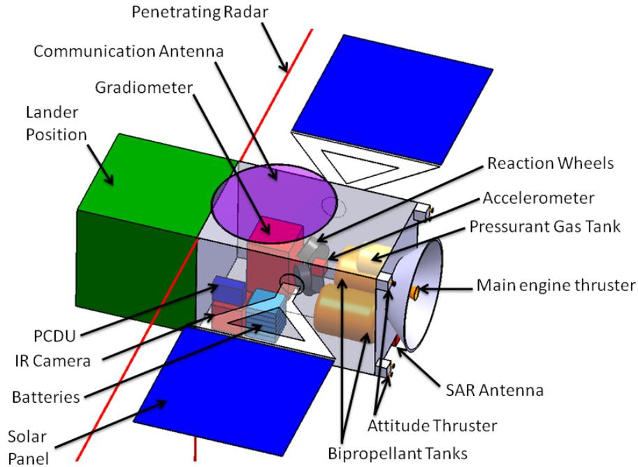
Fig. 5— 3D model of VELOCITÉ orbiter VISAGE.
