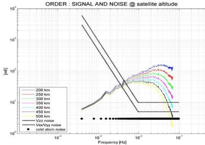
**Figure 2.** Expected gravity signal at different heights compared to noise levels from GOCE and cold atom gradiometer
