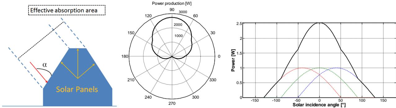
**Figure 9.** The solar panels are located on the top of the spacecraft on the three walls creating roof shape cover (a). This geometry allows heat to be absorbed with respect to the incident angle of the incoming solar flux ( $\alpha$ ). (b) and (c) present the absorbed solar heat flux with respect to the incident angle.
