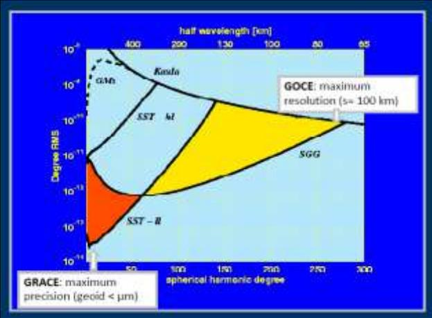
The chart plots Degree RMS (log scale from 10<sup>-14</sup> to 10<sup>-6</sup>) against half wavelength [km] (log scale from 400 to 65) and spherical harmonic degree (log scale from 50 to 3000). Key regions include Kaula (top right), SST (middle), SGG (yellow area), and GRACE/GOCE (bottom left). Annotations specify GRACE maximum precision (geoid < 1 μm) and GOCE maximum resolution (s = 100 km).
