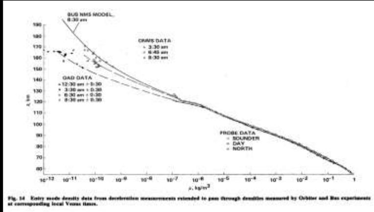
Fig. 14 Entry mode density data from deceleration measurements extended to pass through densities measured by Orbiter and Max experiments at corresponding local Venus times.
