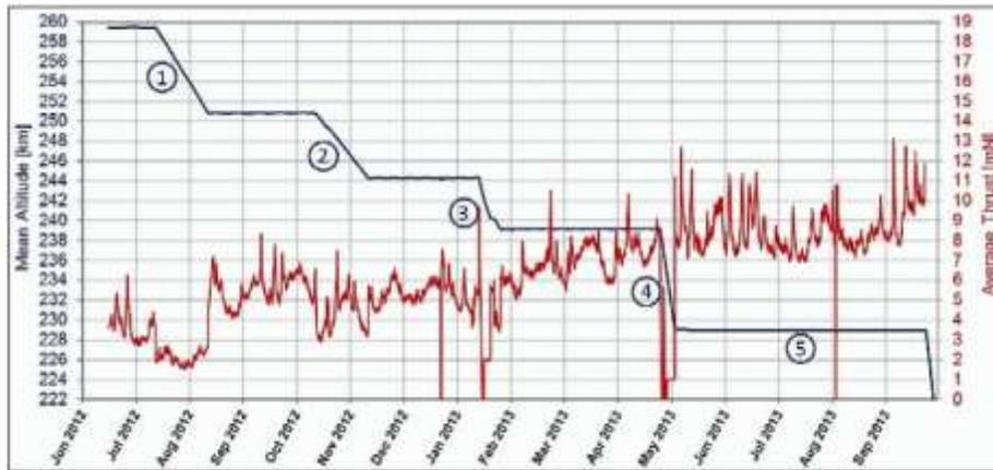
Figure 25: Attitude and average thrust during the low orbit operations campaign (image credit: ESA)
