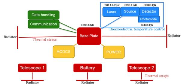
Figure 6: System's thermal control system.
