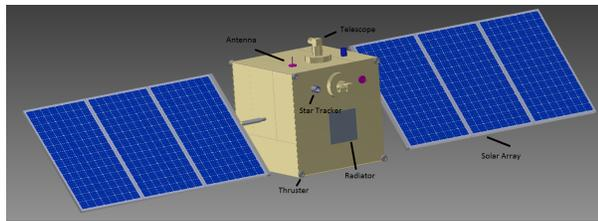
Figure 4: Spacecraft's outer configuration.
