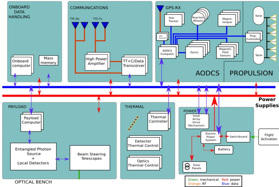
Figure 2: Baseline architecture of the entire satellite system.
