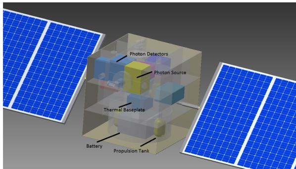
Figure 5: Spacecraft's inner configuration.
