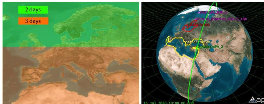
**Figure 2:** Revisit time for different latitudes (left). Orbit with the coastal areas marked.
