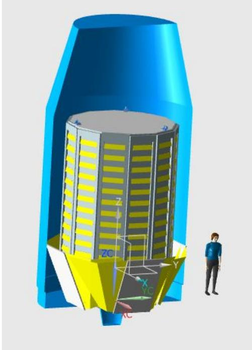
Spacecraft in stowed arrangement compared with the Soyuz fairing usable volume and a human for scale
