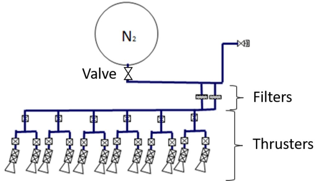
Fully redundant and balanced system
