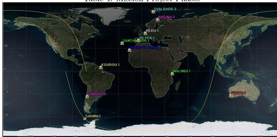
Figure 10: ESTRACK Ground Stations with an overlay of the Orbit.
