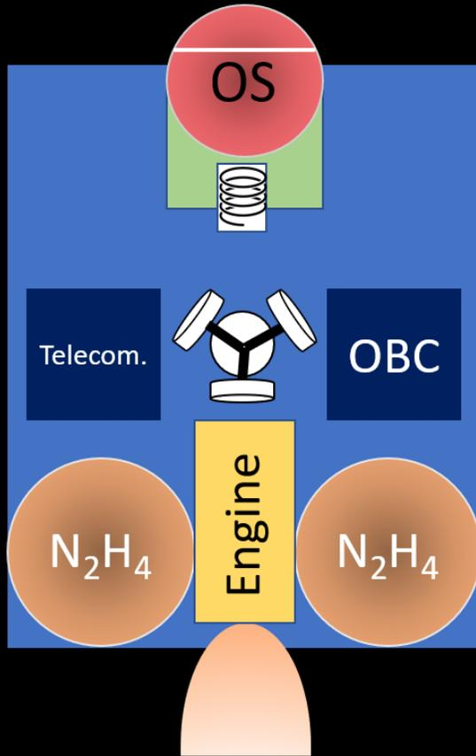
Used for bringing the sample from the surface of Ceres to orbit for docking with the orbiter
