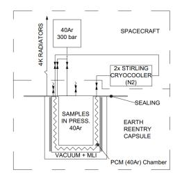
Figure 4: Scheme of the cryocooling system
