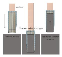
Figure 3: Sampling mechanism
