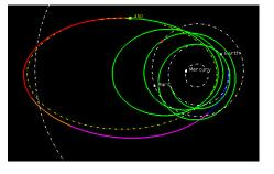
Figure 6: The complete interplanetary trajectory projected on the ecliptic plane. In details: in green the outbound trajectory with a Mars gravity assist at the red dot, in red the operational phase around the comet, in orange the departing maneuver, in purple the inbound cruise and in blue the braking maneuver.
