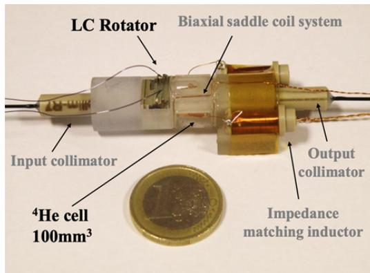
**Figure 2.** Optically pumped He magnetometer.
