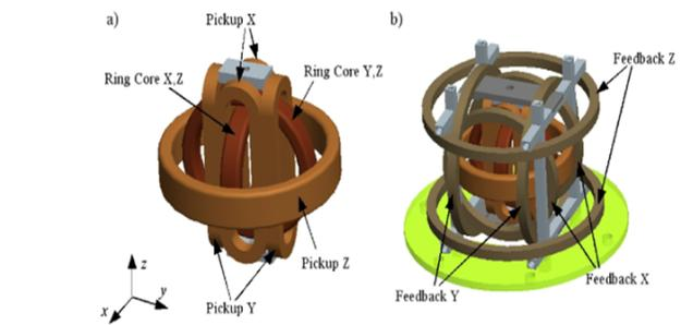
**Figure 3.** A THEMIS miniaturised fluxgate magnetometer.
