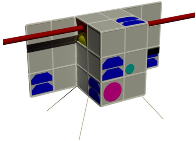
**Figure 4.** Spacecraft structure (back-side). Highlighted elements include: solar cells (blue), S-band antenna (magenta), star tracker (green), deployable booms (brown) and UHF backup antenna (bottom).
