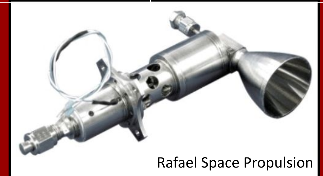
1x 45 N Hydrazine thruster
