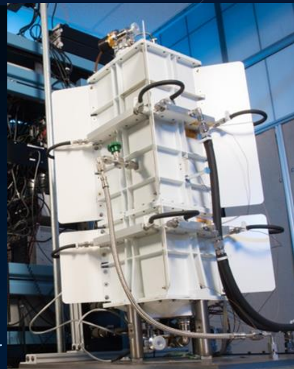
ASRG EU2 test setup, Image Credit: Lewandowski et al. (2016)
