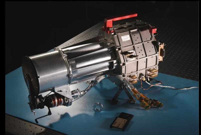
The JANUS (Jovis Amorum ac Natorum Undique Scrutator) VIS-NIR Multi-Band Imager for the JUICE Mission
