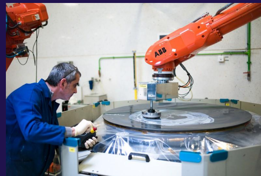
Polishing a telescope mirror. Credits: Christel Sasso / CAPA Pictures / Safran
