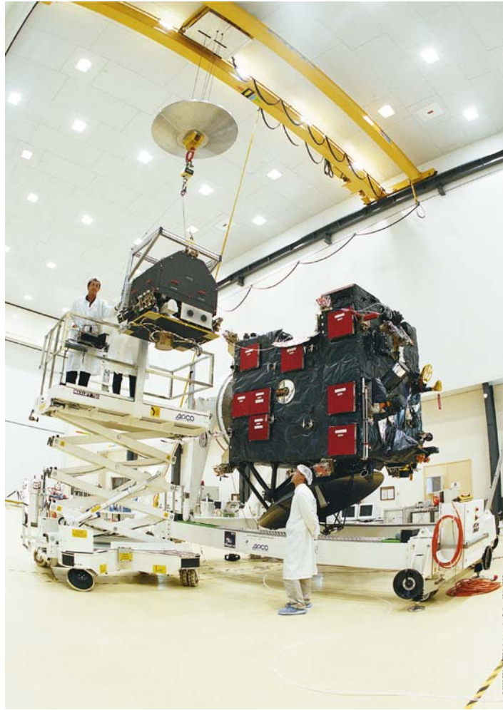
Figure 7. ROSETTA and PHILAE – the lander is attached to the orbiter during integration of the spacecraft. Figure by courtesy of ESA.
