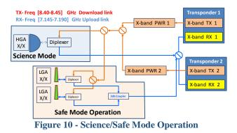
Additionally, the communications subsystem [21] will include hot redundant set of Band X/X transponders and 60W Traveling Wave Tube Amplifier (TWTA) and a RF Distribution Unit (RFDU) with diplexers, 3dB couplers and wave guides to provide the nominal communication with the Earth during different phases of the mission depicted in figure
