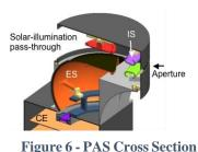
The PAS contains a top hat electrostatic analyser that measures the 3D velocity distribution of protons and alpha particles in the energy range of 0.2 to 20 keV/q with a relative accuracy of 8% (energy), and an
