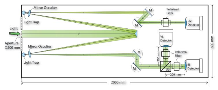
Figure 3: Schematic of the IR/UV Polarimeter
