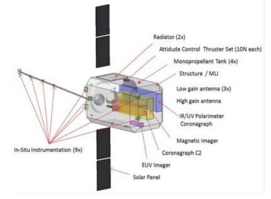
Figure 5: 3D model of the SCE
