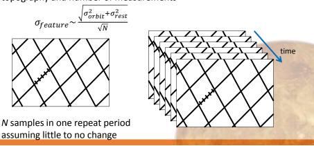
Minimum detectable movement is determined by the quality of topography and number of measurements
