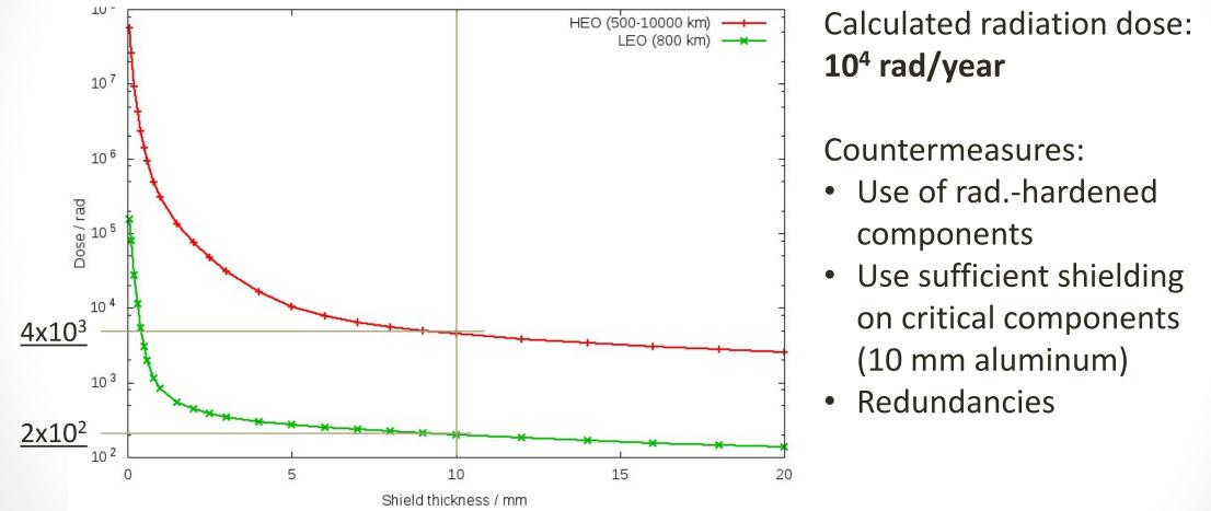
Total radiation dose for two types of orbit (HEO and LEO) computed using SPENVIS (SPace ENVironment Information System)
