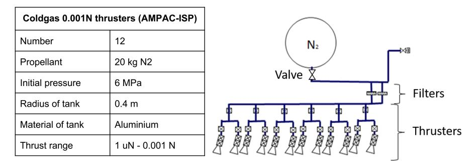
Fully redundant and balanced system Similar system used in EUCLID
