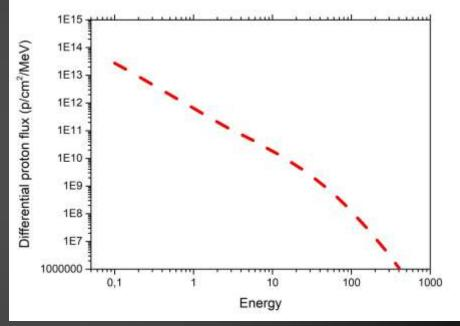
Solar proton flux during comet chasing manoeuvre DDD: 1e11 MeV/g (SPENVIS)
