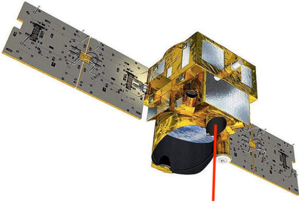
Figure 8: MERLIN active laser remote sensing mission using Airbus/Astrium AstroBus-S spacecraft.
