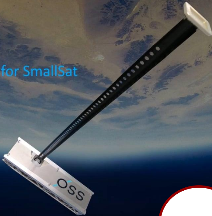
Oxford Space Systems-Astrotube Boom (1.5m)
