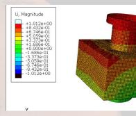
Lateral Frequency: 79.905 Hz Longitudinal Frequency: 217.88 Hz
