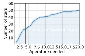
**Figure 7:** Number of stars observable depending on the aperture size assuming an 5 % throughput. Vertical line represents chosen aperture, vertical dashed line shows  $\sim$ 30 % of the total population.
